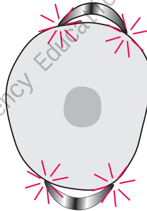
Poorly fitting forcep blades concentrate force at the point of contact
